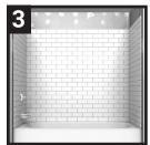
**Step 3:** Install the next row of back and side panels on top of the first row. If done properly, a grout channel will automatically be created that matches the tile pattern. This watertight seam will become invisible even before grouting. The rows of panels can be installed using this same method.
