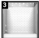
Step 3: Install the next row of back and side panels on top of the first row. If done properly, a grout channel will automatically be created that matches the tile pattern. This watertight seam will become invisible even before grouting. The rows of panels can be installed using this same method as described in Step 1. Always first check the fit of each panel, including the tongue and groove, before adhering to the wall.
