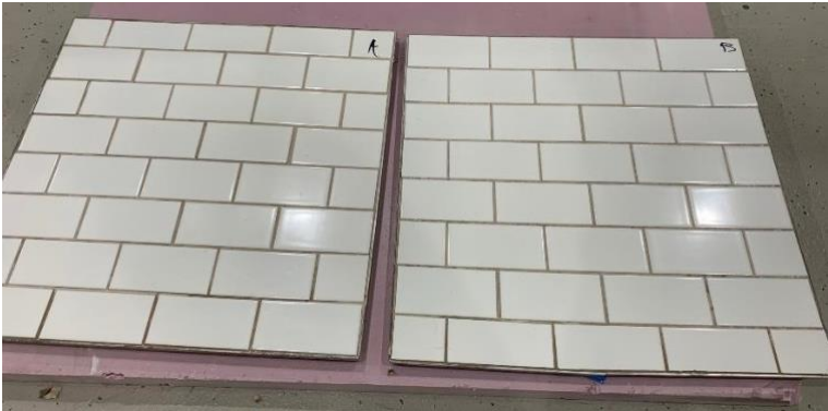
Figure 7. Ceramic Tile Samples - Post 1,344-hour Water Resistance exposure
