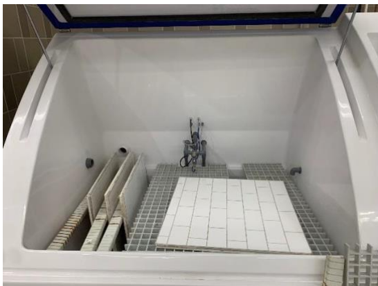
Figure 4. Ceramic Tile, Six3Tile Backsplash and Six3Tile Shower Surround Samples in Salt Fog Machine
