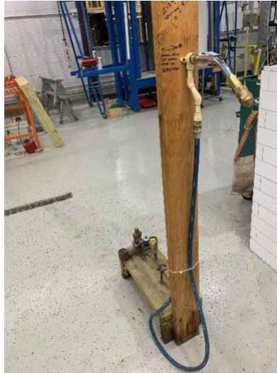
Figure 9. Six3Tile Shower Surround sample undergoing Water Spray Testing
