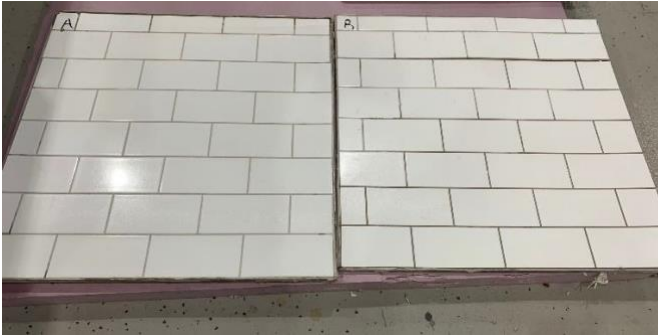
Figure 6. Six3Tile Backsplash Samples - Post 1,344-hour Water Resistance exposure
