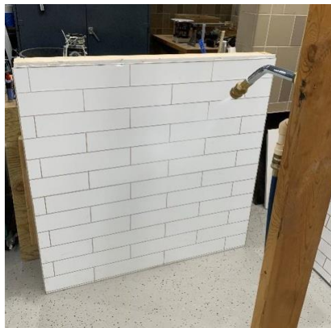
Figure 9. Six3Tile Shower Surround sample undergoing Water Spray Testing
