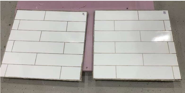
Figure 5. Six3Tile Shower Surround samples - Post 1,344-hour Water Resistance exposure
