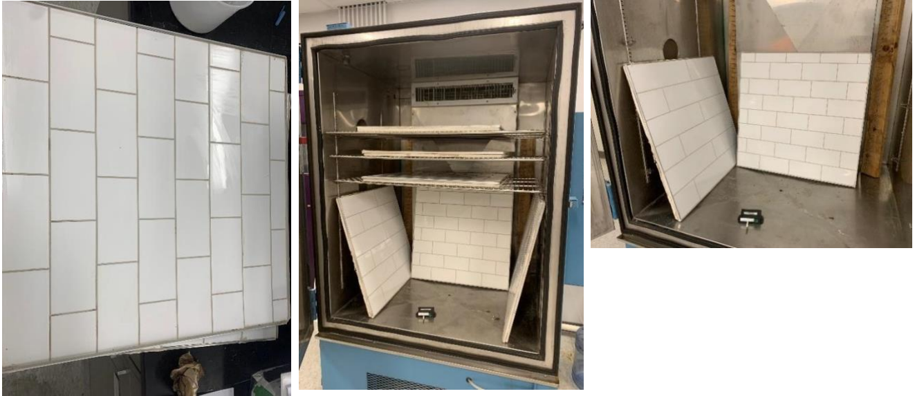
Figure 4. Ceramic Tile, Six3Tile Backsplash and Six3Tile Shower Surround Samples in Environmental Chamber
